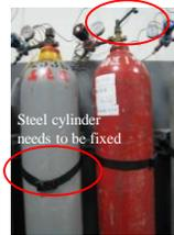
Spare cylinder and empty cylinder should be furnished with cap
